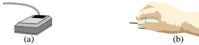
Figure 3: (a) Mouse similar to the original mouse design 20 years ago (b) User's pronated hand grasping a traditionally designed mouse
